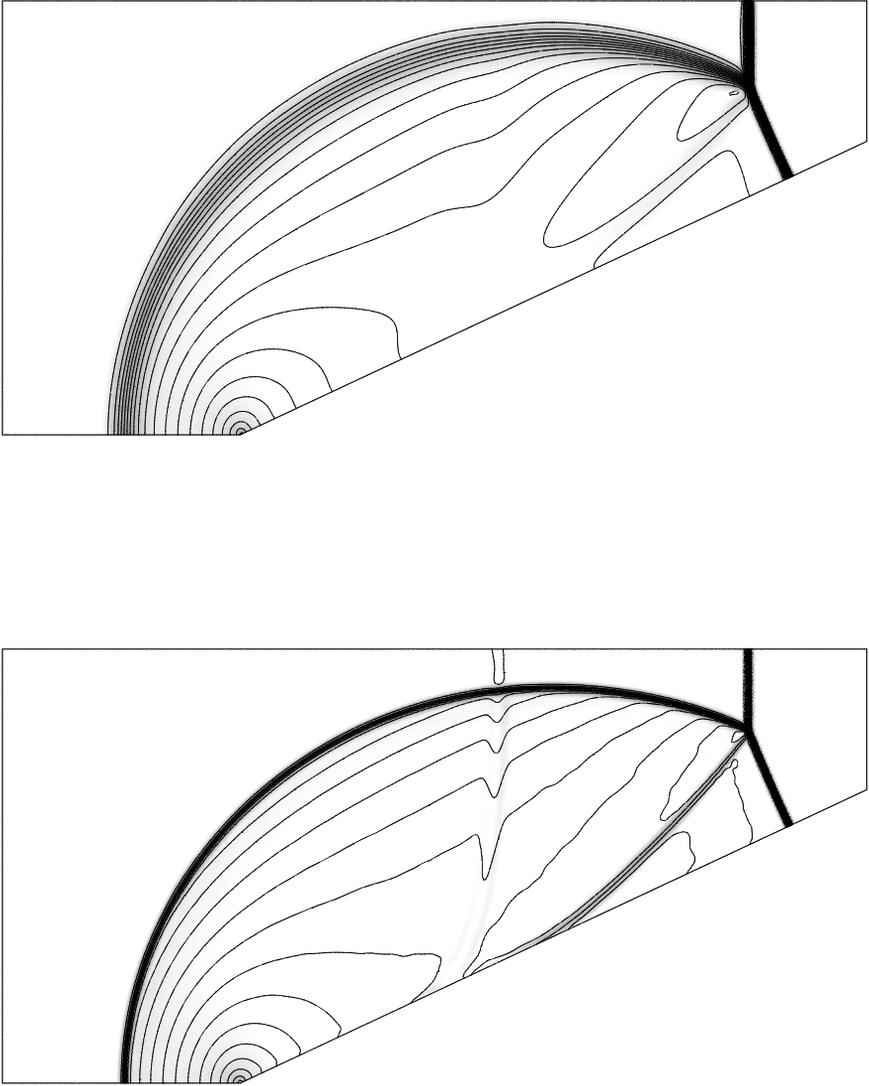
**Fig. 18.11.** Shock reflection problem for shock Mach number 1.7 and wedge angle  $\phi = 25$  degrees. Solution for density on mesh of size  $1/100$ . Top frame: solution from first-order FORCE scheme. Bottom frame: solution from third-order ADER extension of FORCE (Courtesy of Dr. M. Dumbser).
