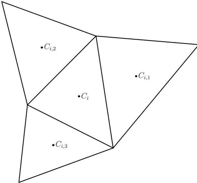
**Fig. 18.8.** Typical unstructured mesh of triangular elements in two space dimensions, called here the primary mesh. Cell  $C_i$  has three neighbours,  $C_{i,1}$ ,  $C_{i,2}$  and  $C_{i,3}$ .
