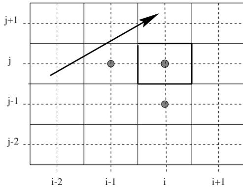
**Fig. 16.4.** Stencil of the Godunov finite volume scheme for the linear advection equation with positive velocity components  $a_1$  and  $a_2$ . The arrow represents the direction of the velocity vector
