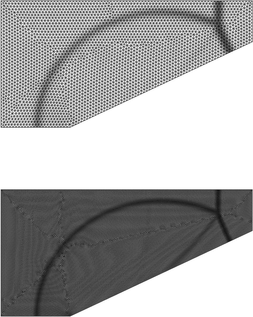
**Fig. 18.10.** Shock reflection problem for shock Mach number 1.7 and wedge angle  $\phi = 25$  degrees. Results from third-order ADER extension of FORCE. Top frame: density contours and unstructured mesh of size 1/20. Bottom frame: density contours and unstructured mesh of size 1/50 (Courtesy of Dr. M. Dumbser).
