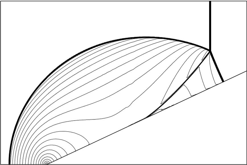
**Fig. 17.9.** Shock reflection problem for  $M_S = 1.7$  and wedge angle of  $\phi = 25$  degrees. Top frame: experimental result (Courtesy of Professor K. Takayama). Bottom frame: density contours from fine regular mesh solution obtained with WAF method and HLLC Riemann solver.
