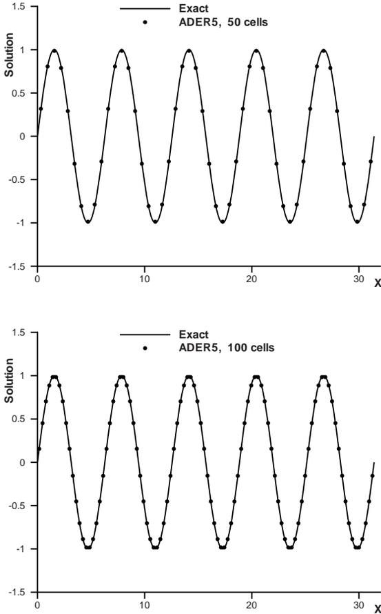
**Fig. 20.4. Advection of smooth profile.** Results from 5–th order ADER scheme (symbols) at time  $t = 1000\pi$  using meshes of 50 and 100 cells, with  $C_{cfl} = 0.95$ . Exact solution shown by full line (Courtesy of Dr. V. A. Titarev).
