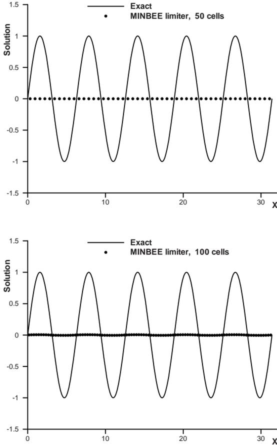
**Fig. 20.2. Linear advection.** Results from TVD scheme with MINBEE limiter (symbols) at time  $t = 1000\pi$  using meshes of 50 and 100 cells, with  $C_{cfl} = 0.95$ . Exact solution shown by full line (Courtesy of Dr. V. A. Titarev).
