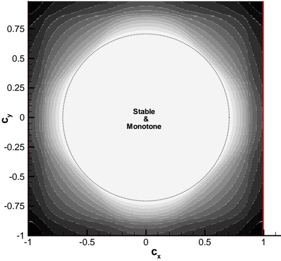
**Fig. 18.6.** Two-dimensional case. Linear stability and monotonicity region in the  $c_x$ - $c_y$  plane.
