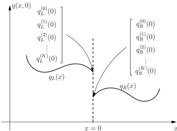
**Fig. 19.3.** Illustration of the initial conditions for the generalized Riemann problem  $GRP_K$  for a single component  $q(x, t)$  of the vector of unknowns  $\mathbf{Q}(x, t)$ . The data  $q_L(x)$  and  $q_R(x)$  are smooth functions away from  $x = 0$  and have one-sided spatial derivatives at  $x = 0$ .
