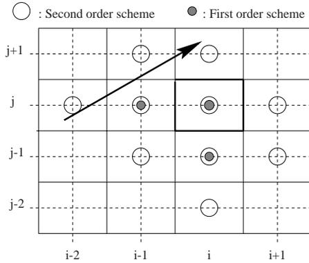
**Fig. 16.5.** Stencil of the MUSCL–Hancock Finite Volume scheme for the linear advection equation with positive velocity components  $a_1$  and  $a_2$ . The arrow represents the direction of the velocity vector. Also shown is the stencil of the first–order version of the scheme
