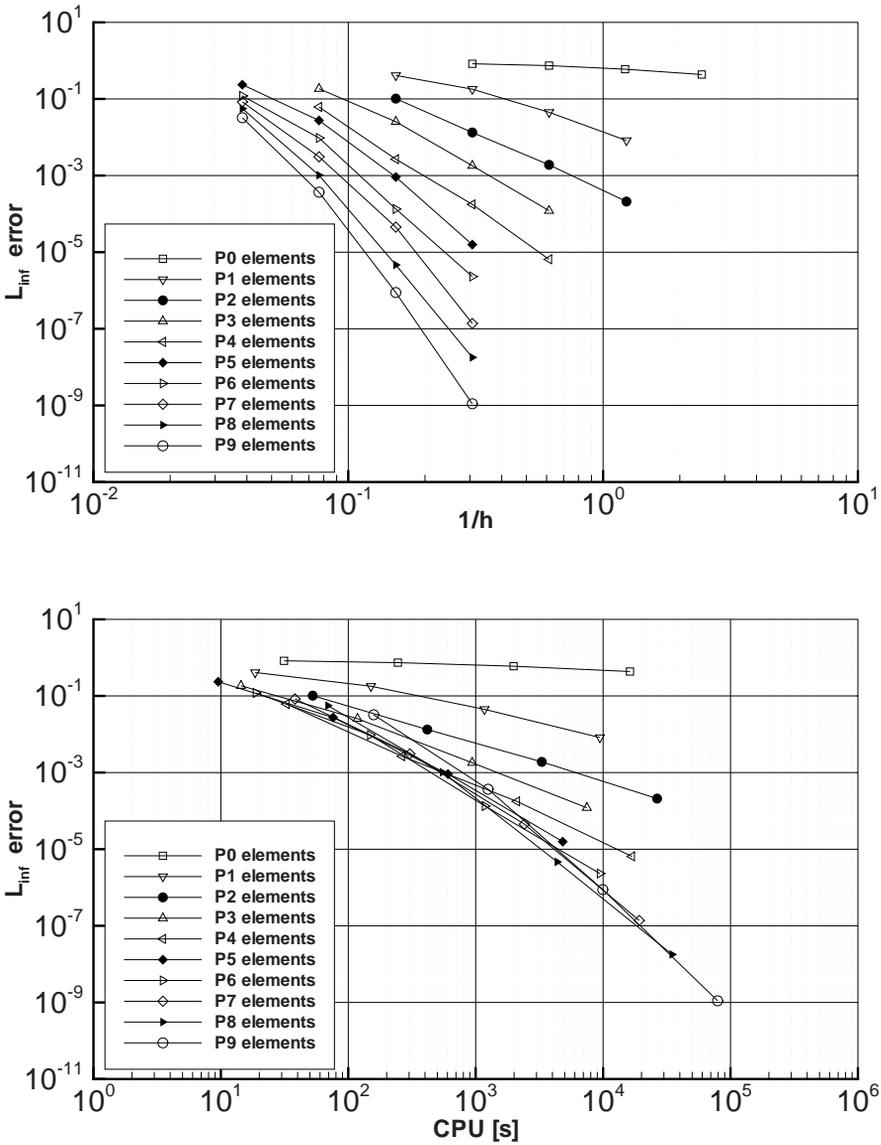
**Fig. 20.5.** ADER discontinuous Galerkin schemes. Error against reciprocal of mesh size (top) and against CPU time (bottom) for schemes of second to tenth order of accuracy in space and time. (Courtesy of Dr. M. Dumbser).
