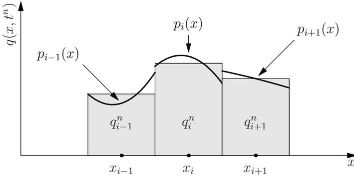
**Fig. 20.1.** Cell averages  $\{q_i^n\}$  define a piece-wise constant distribution  $\{p_i(x)\}$  on each cell  $i$ . Illustration of reconstructed polynomial functions  $p_{i-1}(x)$ ,  $p_i(x)$  and  $p_{i+1}(x)$  in cells  $i - 1$ ,  $i$  and  $i + 1$ , respectively.
