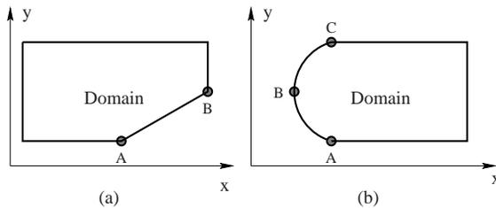
**Fig. 16.11.** Examples of two-dimensional non-Cartesian domains in  $x$ - $y$  space (a) straight segment  $AB$  is not aligned with any of the Cartesian coordinates directions (b) arc  $ABC$  is not aligned with any of the Cartesian coordinates directions
