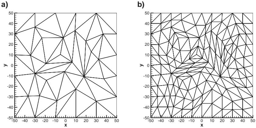
**Fig. 20.6.** Grid topologies for convergence study of ADER discontinuous Galerkin schemes as applied to the linearized Euler equations: (a) very coarse mesh (b) finer mesh (Courtesy of Dr. M. Dumbser).
