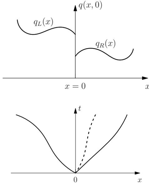
**Fig. 19.2.** The generalized Riemann problem  $GRP_K$  for a typical  $3 \times 3$  hyperbolic system. Top frame shows piece-wise smooth initial condition for a single component  $q$  of the vector  $\mathbf{Q}(x, 0)$ . Bottom frame shows the corresponding wave structure of the solution in the  $x-t$  plane. Characteristics are curved lines.
