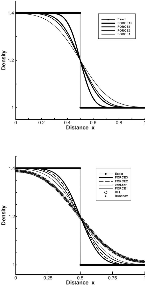
**Fig. 18.4.** Stationary contact test. Comparison of numerical schemes with the exact solution. Top frame: results from the  $FORCE_\alpha$  schemes. Bottom frame: results from  $FORCE_\alpha$  schemes and from the two incomplete Riemann solvers Rusanov and HLL, and from the van Leer Flux Vector Splitting scheme.
