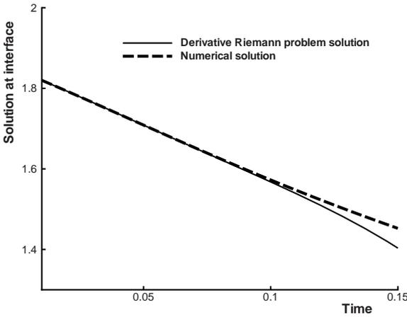
**Fig. 19.5.** Comparison between the reference solution (numerical solution interpolated to the interface position) and the  $GRP_K$  solution to sixth order of accuracy (Courtesy of Dr. V. A. Titarev).
