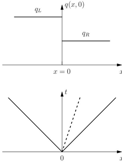
**Fig. 19.1.** The classical Riemann problem for a typical  $3 \times 3$  hyperbolic system. Top frame shows piece-wise constant initial condition for a single component  $q$  of the vector  $\mathbf{Q}(x, 0)$ . Bottom frame shows the corresponding wave structure of the solution in the  $x$ - $t$  plane. Characteristics are straight lines.
