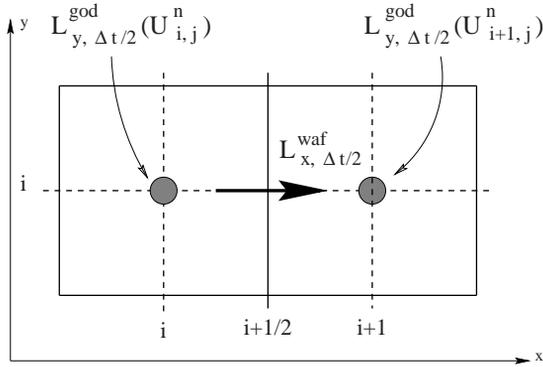
**Fig. 16.9.** Intercell flux  $\mathbf{F}_{i+\frac{1}{2},j}$  is obtained by applying the WAF operator  $\mathbf{L}_{x, \frac{1}{2}\Delta t}^{waf}$  in the  $x$ -direction to modified data in cells  $(i, j)$  and  $(i+1, j)$ . Modified data is obtained by applying the Godunov operator  $\mathbf{L}_{y, \frac{1}{2}\Delta t}^{god}$  in the  $y$ -direction to initial states  $\mathbf{U}_{i,j}^n, \mathbf{U}_{i+1,j}^n$
