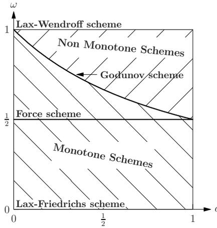
**Fig. 18.1.** Weighted FORCE-type fluxes defined as convex averages of the Lax–Friedrichs and Lax–Wendroff fluxes in the  $c - \omega$  plane. Here  $c$  is Courant number and  $\omega$  is a weight, whose constant values  $0, \frac{1}{2}$  and  $1$  reproduce the Lax–Friedrichs, FORCE and Lax–Wendroff fluxes;  $\omega = 1/(1 + |c|)$  reproduces the Godunov upwind method.
