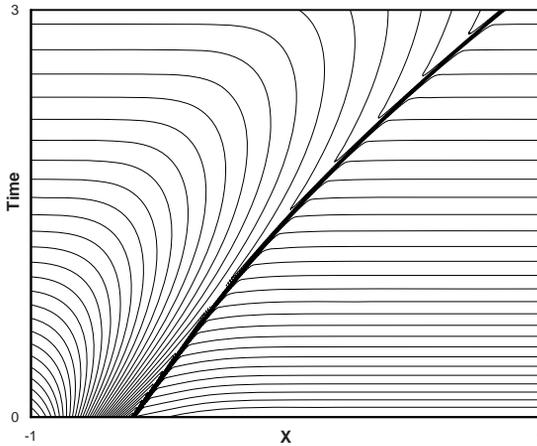
**Fig. 19.4.** Contour plot of the numerical solution of the generalized Riemann problem for the inviscid Burgers equation with a non-linear source term. The main feature of the solution is an accelerating shock wave that propagates to the right (Courtesy of Dr. V. A. Titarev).
