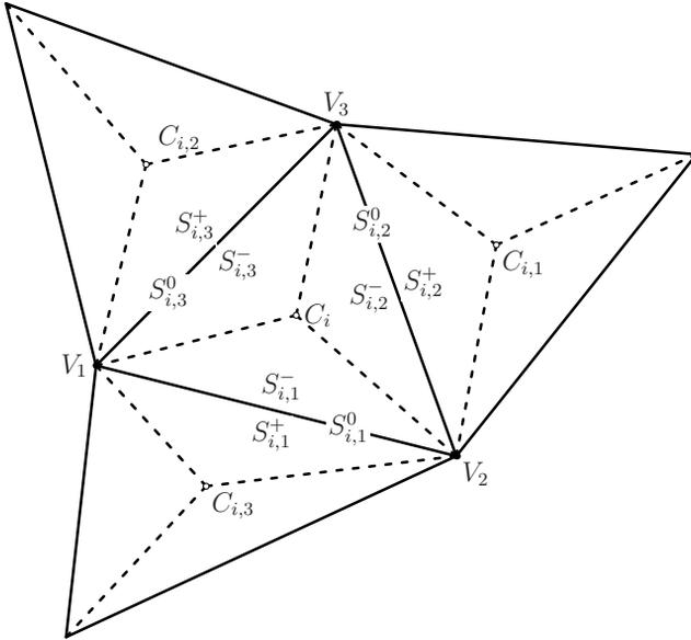
**Fig. 18.9.** Primary mesh of triangular elements  $C_i$  and edge-based staggered mesh of elements  $S_{i,j} = S_{i,j}^- \cup S_{i,j}^+$ ,  $j = 1, 2, 3$ , and cell edges  $S_{i,j}^0 = S_{i,j}^- \cap S_{i,j}^+$ ,  $j = 1, 2, 3$ .
