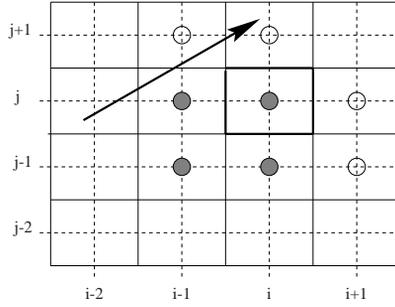
**Fig. 16.8.** Stencil of the second-order WAF finite volume scheme for the two-dimensional linear advection equation with positive  $a_1$  and  $a_2$ . Compare with stencil of first-order scheme of Fig. 16.7
