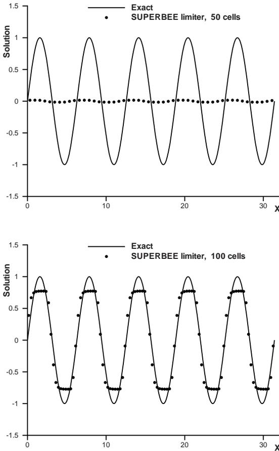
**Fig. 20.3. Linear advection.** Results from TVD scheme with SUPERBEE limiter (symbols) at time  $t = 1000\pi$  using meshes of 50 and 100 cells, with  $C_{cfl} = 0.95$ . Exact solution shown by full line (Courtesy of Dr. V. A. Titarev).
