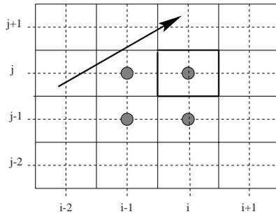
**Fig. 16.7.** Stencil of the first-order WAF finite volume scheme (identical to the CTU scheme of Colella) for the two-dimensional linear advection equation with positive  $a_1$  and  $a_2$ . The arrow indicates the direction of the velocity vector
